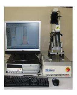
Figura 17. Texturometro Stable Micro Systems modelo Texture Analyzer– XT plus
